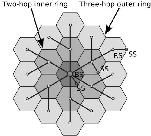
Figure 1: Three-hop hexagonal relay topology.
